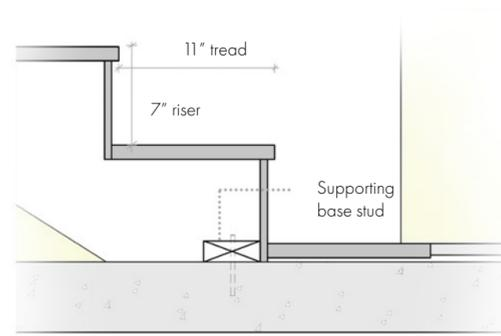
DETAIL B - Floor slab and stringer beam connection
