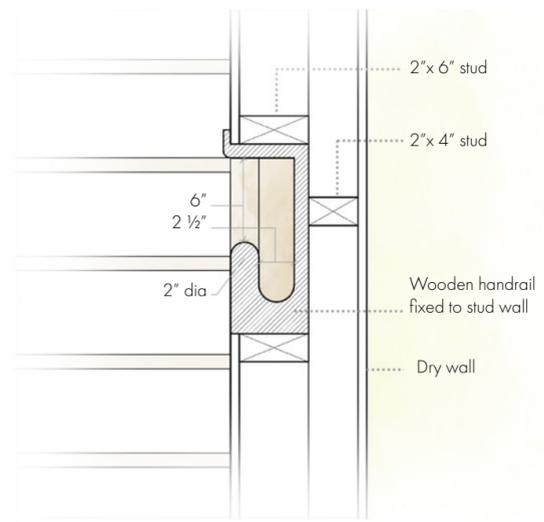
DETAIL D - Handrail detail
